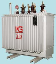
315 kVA, 11/0.4 kV, NLTC -7 Tap (Aluminium winding Type)
