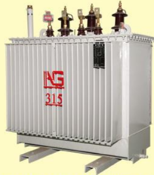
315 kVA, 11/0.4 kV, NLTC -7 Tap (Aluminium winding Type)
