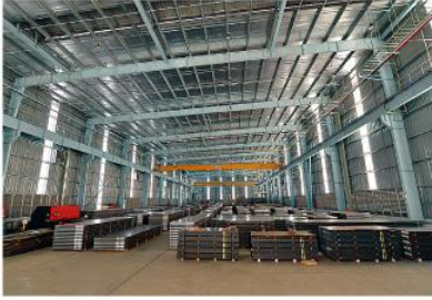
Cut sheet processed from a coil shape to a flat. The company provides stable quality to Myanmar with materials made in Japan.
