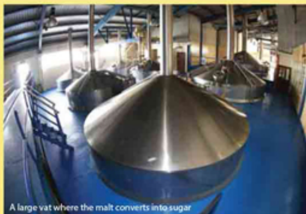
A large vat where the malt converts into sugar
